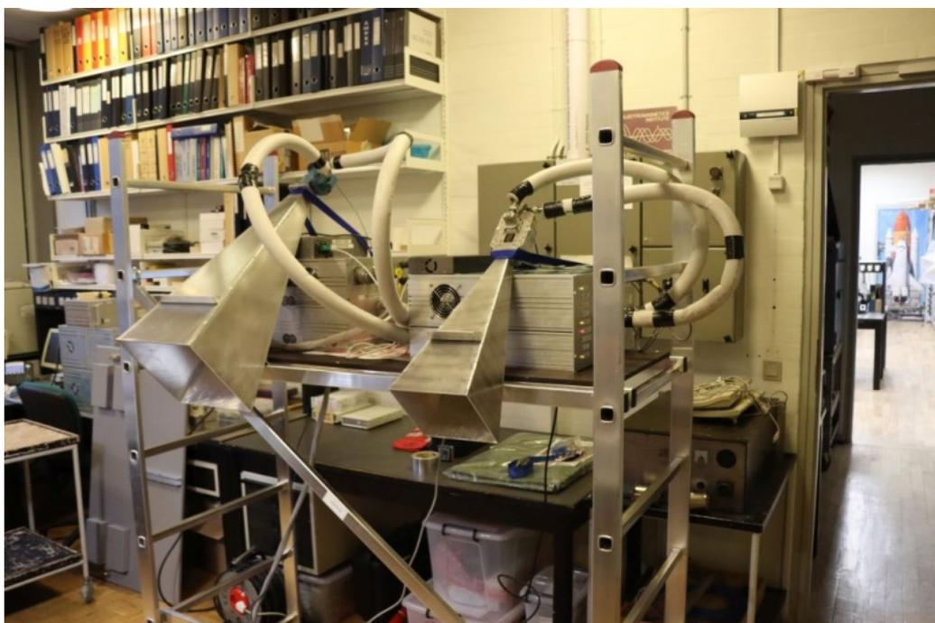
Figure 5-1 – Scaffold accommodating EMIRAD-C (left) and EMIRAD-X (right)
