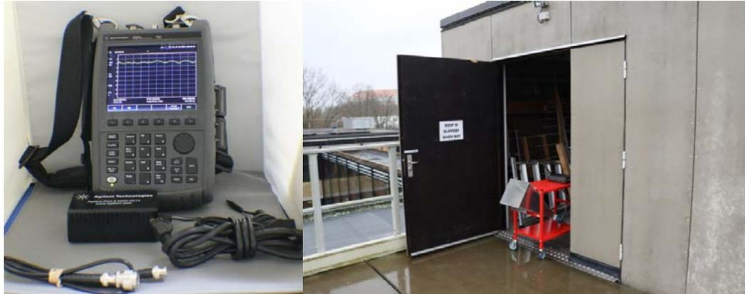
Figure 4-6 – Vector Network Analyzer (left) and antenna looking into free space (right)
