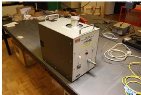
Figure 3-3 – Cryostat containing a matched load
